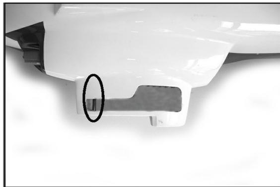
Insert the 4x55mm Carbon Rods into the specific position of the Gun Housing and secure it with glue. (This is used to prevent further retraction of the Retract System.)
