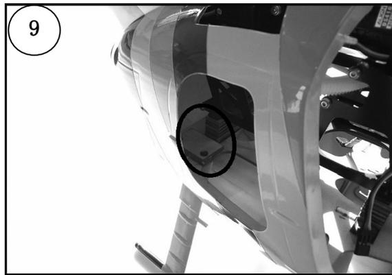
Put the wood fixing block insert the Plywood slot.
