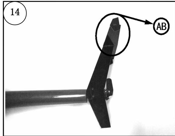
Glue the Horizontal Stabilizer on the Vertical Stabilizer like the picture. (Make sure it is balance.)
