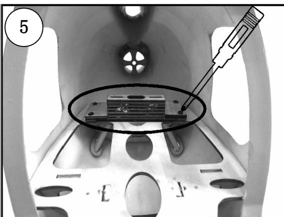
Stick the wood pieces on the Backplane with Combination self-Tapping Screw 2x10mm.
