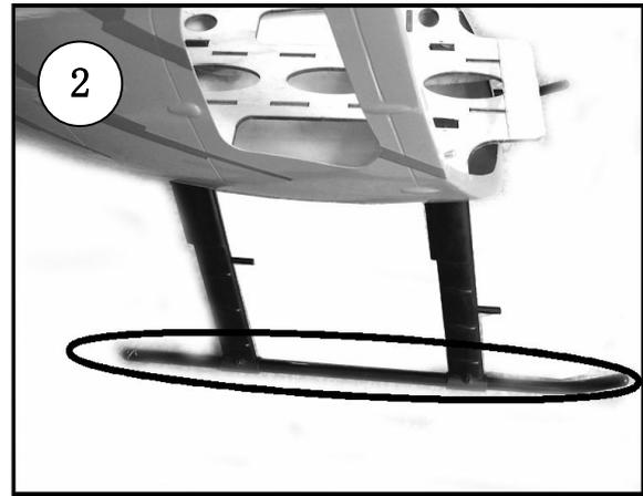
Insert the skid pipes into the front and rear landing skids as illustration.
