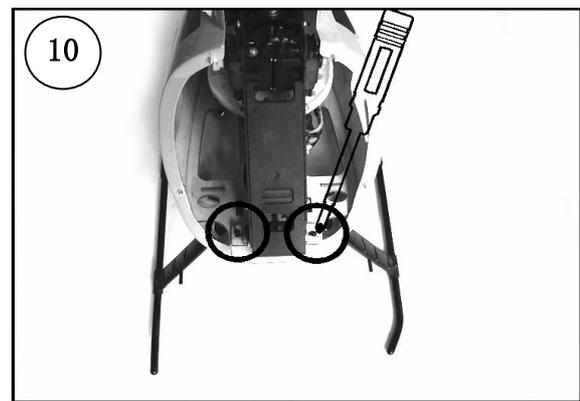
Stick the wood pieces under the center of the body. (Combination self-Tapping Screw 2x10mm)
