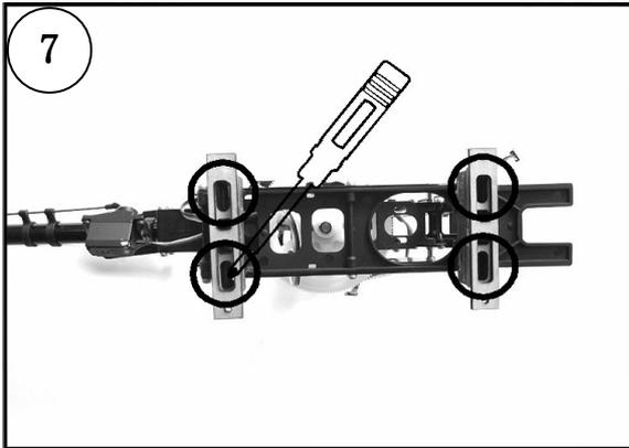
Stick the Wood pieces under the Body. (Hex Cap Screw 2x25mm x4; Nuts 2x5mmx4 ; washer  $\varnothing 2.5$ x  $\varnothing 5$ x0.5mmx4)
