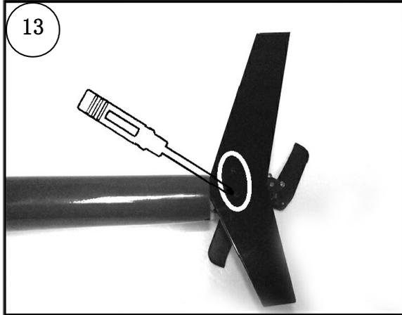
Stick and make sure the Vertical Stabilizer alignment the tail. (Hex Cap Screw 2x18mm; Washer  $\varnothing$  2.5x  $\varnothing$  5x0.5mm)
